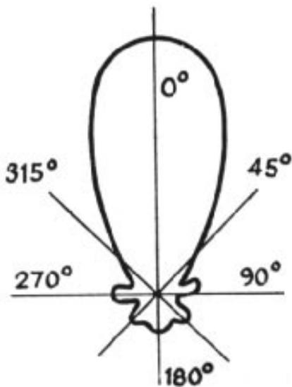
Fig. 6 - Measured radiation pattern for the lowest frequency band (14 MHz) of a 12-element 13-30 MHz log-periodic dipole array. For its design parameters,  $\tau = 0.9$  and  $\sigma = .05$ . The measured front-to-back ratio is 14.4 dB at 14 MHz, and increases to 21 dB at 28 MHz.
